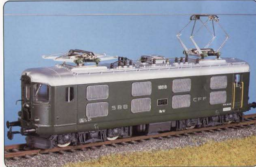
Re 4/4 Series 1 No. 225 AC, No. 226 DC. This locomotive which is equipped with multiple-unit control was specially designed for shuttle-train traffic but could also be used for express trains over flat terrain. It is still giving faithful service on branch lines. Entered service 1946-1948, 2520hp, 58 tons, 125km/hr.
