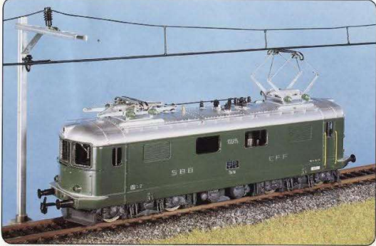
Re 4/4 Series 2 No. 220 AC, No. 221 DC. Together with its forerunner and sister model (No. 225/226), this first Bo-Bo locomotive was considered a revolutionary innovation in Swiss locomotive construction. It was the first graceful and elegant-looking express-train locomotive. Entered service 1950/51, 2520hp, 58 tons, 125km/hr.
