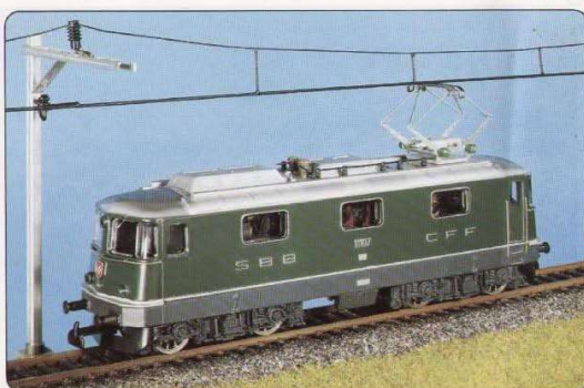
Re 4/4 1 No. 160 AC, No. 161 DC. Swiss Federal Railways (SBB) put the first locomotive of this type into service in 1967. These Re 4/4 1 with a diamond pantograph and still with a shunter locomotive body are still in service. 6320hp, 80 tons, 140km/hr.
