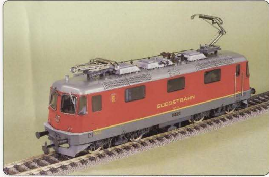
Re 4/4 #508 No. 270 AC, No. 271 DC, one of the 3 Re 4/4s operated by the South-Eastern Railway (Südostbahn) is numbered 44 and named «Pflätkon». The SOB operates between Romanshorn and Lucerne, working in part over Bodensee-Lögnenberg Railway (BL) lines. The figure 1 after Re 4/4 indicates that it is geared for operating on mountainous routes.
