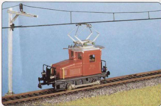
Te 101 No. 131 DC. This shunter handles day-to-day shunting jobs and engineering movements at most Swiss stations. Entered service 1941-45, 340hp, 28 tons, 60km/hr.
