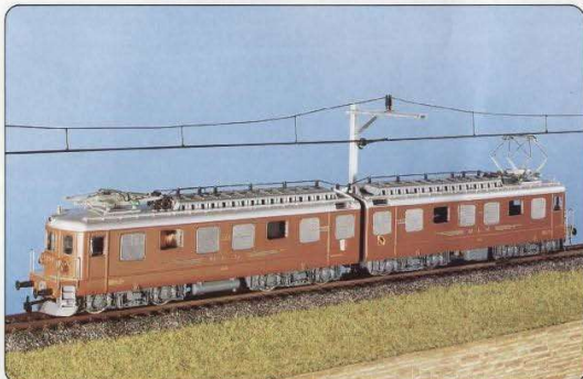
Ae 8/8 BLS No. 240 AC, No. 241 DC. This locomotive, which is the strongest possessed by the Berner-Lötschberg-Simplon Railway, is used mainly for heavy freight trains and especially for the famous Motorail across the Alps. Entered service 1959, 8800hp, 160 tons, 125km/hr. Ae 8/8 BLS No. 242 AC, No. 243 DC. Type with 2 engines, most powerful locomotive in scale HO from the world.
