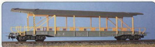
BLS car transport carriage No. 370 AC, No. 371 DC. The characteristic car transport carriages with their protective roofs against falling stones are a familiar sight for many tourists.
