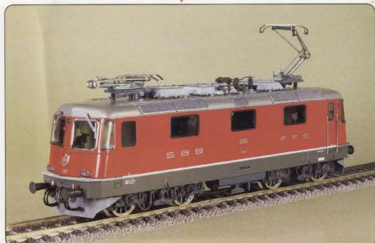
Re 4/4 1 new finish No. 165 AC, No. 166 DC. The latest finish for the Re 4/4 1 , with 2 pantographs, rectangular halogen headlights and the new red livery. The HAG model is also a completely new construction. Entered service 1984, 6320hp, 80 tons, 140km/hr.
