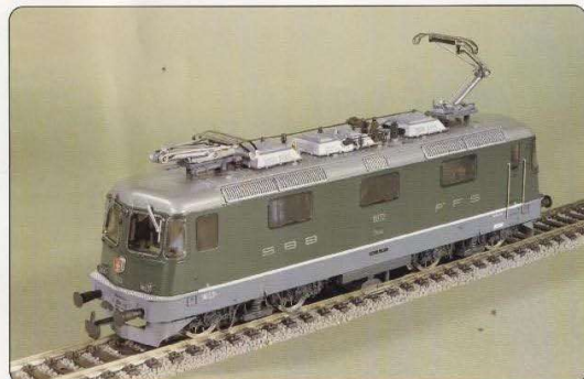
Re 4/4 1 No. 167 AC, No. 168 DC. The first 7 of the latest Re 4/4 1 delivered to the SBB in 1984 were still finished in the old green livery, and will also stay like this until their first general overhaul. Entered service 1984, 6320hp, 80 tons, 140km/hr.
