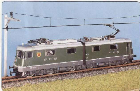
Re 6/6 No. 200 AC, No. 201 DC. 85 of these locomotives were ordered in all, but only the first two prototypes were built in two-part form. The Re 6/6 is one of Europe's most powerful locomotives and is mainly used to haul superheavy trains on the St. Gotthard line. Entered service 1972, 10500hp, 120tons, 140km/h. This model will also be available in red livery in due course!
