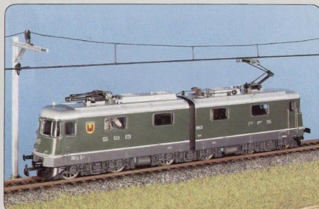
Re 6/6 No. 200 AC, No. 201 DC. 45 of these locomotives were ordered in all, but only the first two prototypes were built in two-part form. The Re 6/6 is one of Europe's most powerful locomotives and is mainly used to haul super-heavy trains on the St. Gotthard line. Entered service 1972, 10 600 hp, 120 tons, 140 km/hr.
