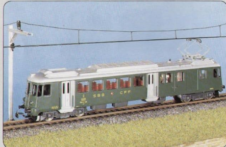
SBB self-propelled coach No. 150 AC, No. 191 DC. Made up to form shuttle trains, these self-propelled coaches are used to transport passengers and their luggage between suburban stations and terminals all over Switzerland. 1600 hp, 57 tons, 110 km/hr.
