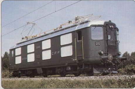
Re 4/4 Series 1 No. 225 AC, No. 226 DC. This locomotive which is equipped with multiple unit controls was especially designed for shuttle train traffic but could also be used for express train over flat terrain. It is still going faithful service on branch lines. Entered service 1946-1948, 2520hp, 56t, 125km/h.
