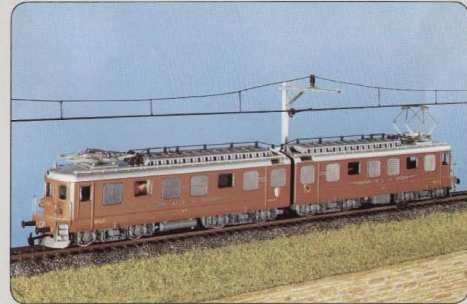
Ae 8/8 BLS No. 240 AC, No. 241 DC. This locomotive which is the strongest possessed by the Bern-Lötschberg-Simplon Railway, is used mostly for heavy freight trains and especially for the famous Motorail across the Alps. Entered service 1959, 8800 hp, 160 tons, 125 km/h.
