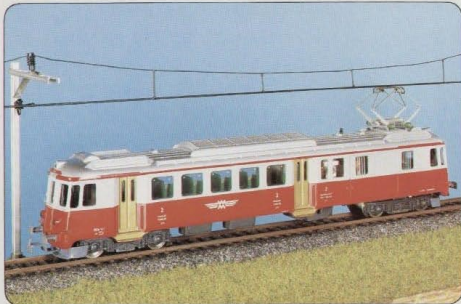
WM self-propelled coach No. 250 AC, No. 251 DC. The route of this normal-gauge private railway connecting Wohlen with Mieselschwandlen is only 8,253 km long. Normally one self-propelled coach type BD e 4/4 is used on this route. In peak hours another driving trailer is attached. Entered service 1968, 1500 hp, 63 tons, 100 km/h.
