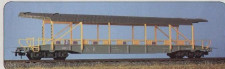
BLS car transport carriage No. 370 AC, No. 371 DC. The characteristic car transport carriage with their protective roof against falling stones are a familiar sight for many tourists.
