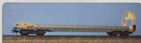
BLS ramp carriage No. 375 AC, No. 376 DC. The first and the last carriage of each car transport conveyer is a ramp carriage for driving on and off.
