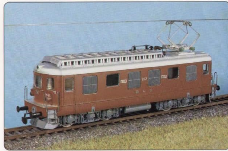
Re 4/4 BLS No. 182 AC, No. 183 DC . This «Bern-Lötschberg-Simplon Railway» locomotive type is the forerunner of the Re 4/4 (180/181). Of the 8 originally delivered, 4 were rebuilt in 1965-1966 into 2 Ae 8/8s. Introduced 1944, 4000hp, 80 tons, 120km/hr.
