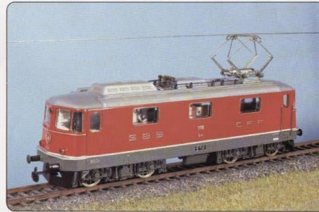
Re 4/4 1 No. 162 AC, No. 163 DC. Since mid-1984, older SBB locomotives, such as the Re 4/4 1 of the first series, are also being repainted in red when they undergo their next general overhaul. Here is locomotive No. 1115 which has already been repainted. Entered service 1967/68, 6320hp, 80 tons, 140km/hr.
