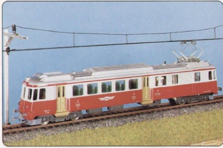
WM self-propelled coach No. 250 AC, No. 251 DC. The route of this normal-gauge private railway connecting Wohlen with Meereschwenden is only 8.233km long. Normally one self-propelled coach type BDe 414 is used on this route. In peak hours another driving trailer is attached. Entered service 1966, 1500hp, 63tons, 100km/hr.
