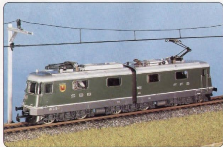
Re 6/6 No. 200 AC, No. 201 DC . 45 of these locomotives were ordered in all, but only the first two prototypes were built in two-part form. The Re 6/6 is one of Europe's most powerful locomotives and is mainly used to haul superheavy trains on the St. Gotthard line. Entered service 1972, 10800hp, 120 tons, 140km/hr. This model will also be available in red livery in due course!
