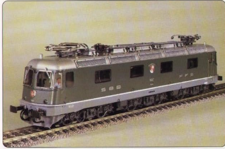
Re 6/6 No. 205 AC, No. 206 DC . The 43 locomotives with non-articulated bodies delivered to the SBB for the St. Gotthard line from 1975 on carry the names and coats of arms of places in Switzerland which are of special importance for transport or have a special link with the railway. This model is supplied with a different number and nameplate on each side. Entered service 1975-1979, 10600hp, 120 tons, 140km/hr.
