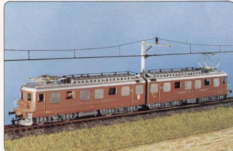
Re 8/8 BLS No. 240 AC, No. 241 DC. This locomotive, which is the strongest possessed by the Berner-Lötschberg-Simplon Railway, is used mainly for heavy freight trains and especially for the famous Motorail across the Alps. Entered service 1959, 8800hp, 160 tons, 125 km/hr.
