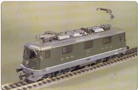
Re 4/4 1 No. 167 AC, No. 168 DC. The first 7 of the latest Re 4/4 1 s delivered to the SBB in 1984 were still finished in the old green livery, and will also stay like this until their first general overhaul. Entered service 1984, 6320hp, 80 tons, 140km/hr.
