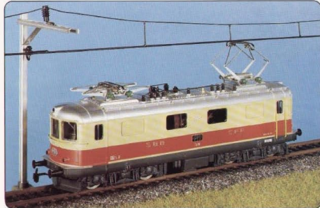
Re 4/4/1 TEE No. 230 AC, No. 231 DC. Of the 24 type Re 4/4 model, only four were selected to be repainted as TEE engines. They haul international expresses right through Switzerland. Entered service approx. 1963-1965, 2520hp, 58 tons, 125 km/hr.
