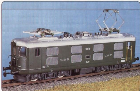
Re 4/4/1 Series 1 No. 226 AC, No. 226 DC. This locomotive which is equipped with multiple control was specially designed for shuttle-train traffic but could also be used for express trains over flat terrain. It is still giving faithful service on branch lines. Entered service 1946-1948, 2520hp, 58 tons, 125 km/hr.
