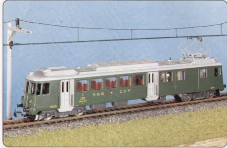
SBB self-propelled coach BDe 4/4 No. 150 AC, No. 151 DC. Made up to form shuttle trains, these self-propelled coaches are used to transport passengers and their luggage between suburban stations and terminals all over Switzerland. 1600hp, 37 tons, 100km/hr.
